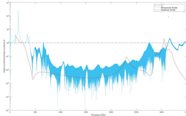
Aluminum alloy load carrying phononic crystal, produced by additive manufacturing (left) and transmissibility curves (calculated and measured) of the device. A wide region of very low transmissibility (attenuation of the order of 99%) is observed between approximately 400Hz and 3000Hz. This property allows, for example, to decouple the vibration of motors from the surrounding environment.
