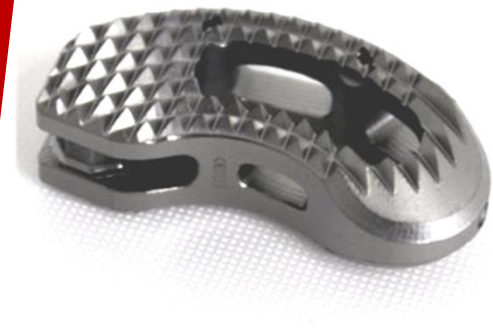
T-PAL PEEK spinal spacer (Ti, HiPIMS coated at Empa)
