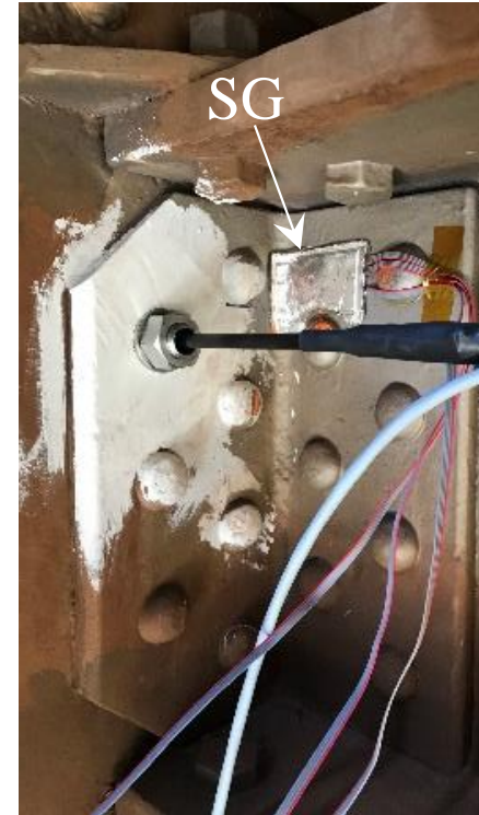
Rosette strain gauge for the short-term measurements
