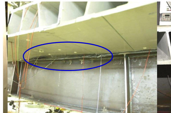
Failure of adhesive bond
