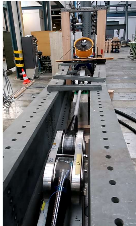
Fatigue experiments in 2020 on CFRP hangers
