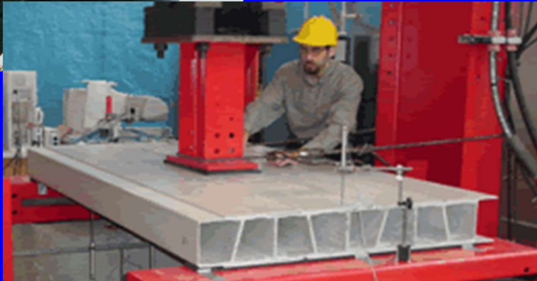
Laboratory testing of an FRP bridge deck panel
