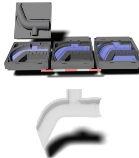
Fig.1 top: 3D-rendering of the mold at different stages of filling and the overflow in the right depiction. Bottom: 3D model of one representative part.
