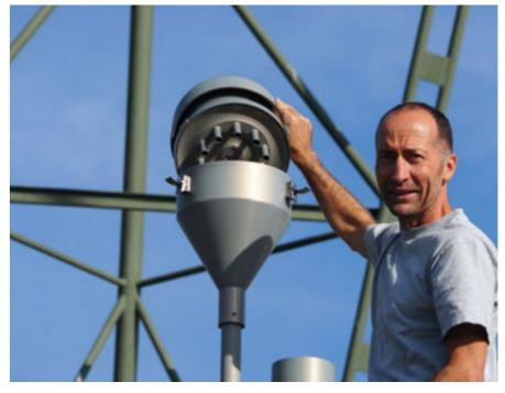
The fine particulate matter is collected in so-called impactors on the roof of the former control center at the foot of the tower. Christoph Hüglin (left) and Stefan Bugmann not only analyze the reading transmitted online, but also the contents of the filters.
