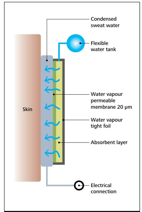
Function diagram: Thanks to a water reservoir, the electrode always remains moist and yields reliable data.
