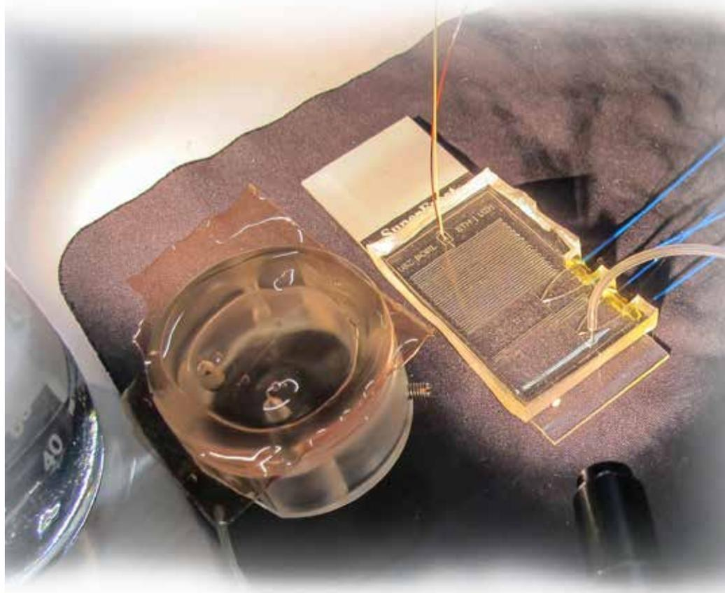
Initially, glucose molecules diffuse through the membrane from the skin (left) before enzymes are added and the solution is pumped through the microfluidics chip (right). By means of fluorescence measurement the glucose concentration in the blood can be calculated.
