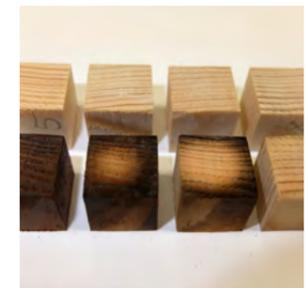
From left to right: wood samples with rising limestone concentrations next to an untreated control sample.
