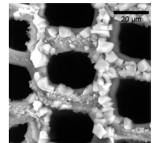
The limestone crystals are clearly visible in the cell walls.
