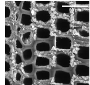
Hybrid wood under the electron microscope: using the production technique with ester and calcium chloride, the limestone crystals are embedded in the cell walls.
