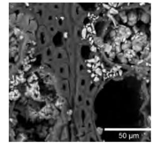
For an alternative technique, which Vivian Merk also developed, two solutions are used alternately. Here, the limestone crystals are embedded within the cells.
