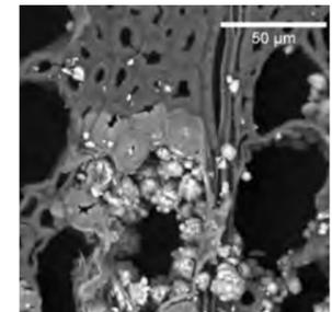
Method 2: limestone crystals are embedded within the cells.
