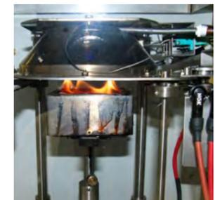
All samples are tested at a defined distance from the flame in flame tests in the lab.
