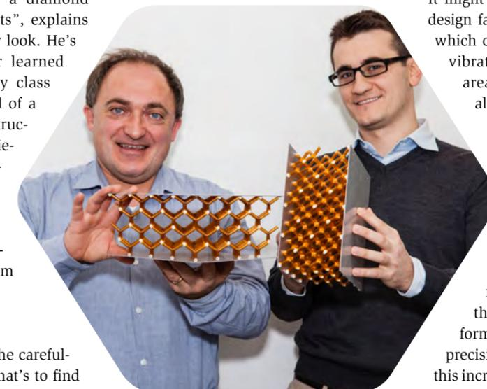
at all. The researchers had discovered what is known as a “band gap” in the macrocrystal – a property that also plays a central role in semiconductor technology. Within this band gap, the macrocrystal does not transmit any vibrations.
