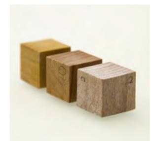
From left to right: untreated wood, treatment with one solution, treatment with two solutions alternately.
