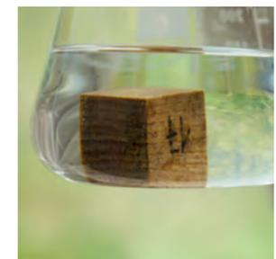
Immersing the sample in the ester solution for several hours ensures that it soaks right through to the cells.
