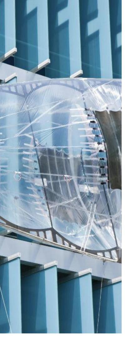
An example of a smart material: In Empa's Blimp, electroactive polymers (black area) stretch or contract when an applied voltage is turned on and off. The resulting flapping of the tail fin propels the airship forward.
