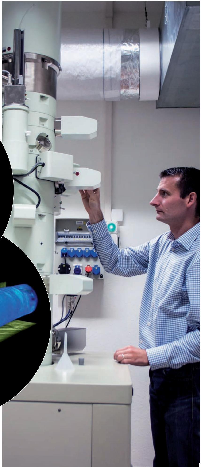
Rolf Erni working with the scanning transmission electron microscope: the individual images are put together electronically. Top: 3-D view of the type of lithium iron phosphate particle that occurs in lithium-ion batteries. Bottom: Opalinus clay, a potential barrier material for nuclear waste.
