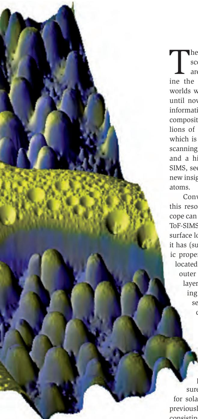
A typical image from the 3-D NanoChemiscope showing the atomic structure of a surface: the instrument provides information about the chemical composition of the upper layers.
