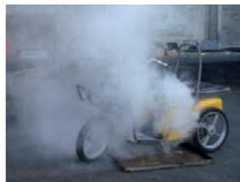
Short circuit on Li-ion-batteries 24
