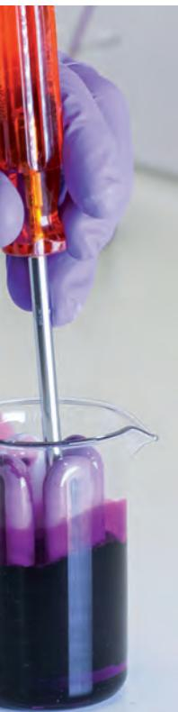
How Empa measures the amount of mercury in energy-saving lamps: The lamp is submerged in a potassium permanganate solution and the glass bulb is broken. Because of the pressure difference, the solution shoots into the lamp and washes out the gaseous mercury. The glass is then ground into a powder and the attached amounts analyzed separately.
