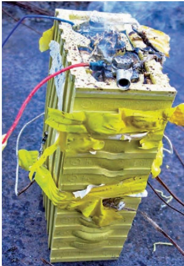
This is what a lithium iron phosphate battery looks like after it has been pierced by a nail. The internal short-circuit makes the battery heat up. Gas escapes from the top; the casing becomes soft and bulges in several places. But the battery does not burn.
