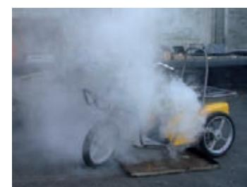
Short circuit on Li-ion-batteries 24
