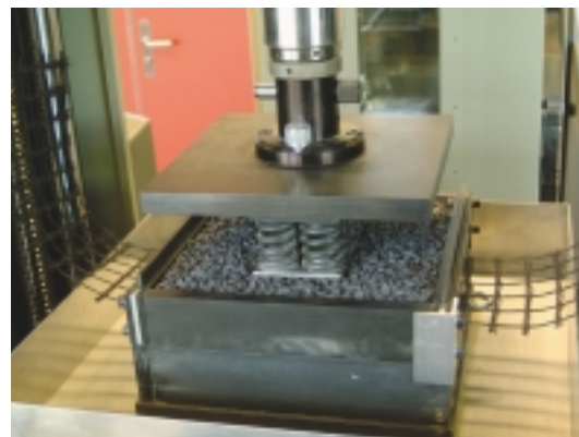
Fig. 1: Test equipment for simulating damage during installation.
