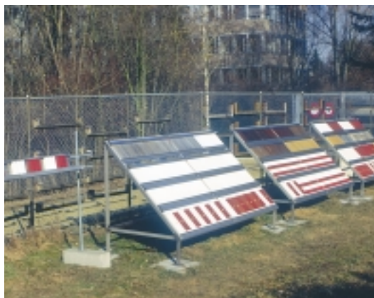
Fig. 3: Conventional natural exposure test on a 45° plane facing South.
