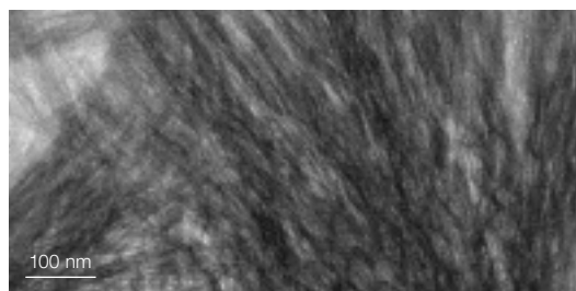
Fig. 3: TEM brightfield imaging (FIB preparation) showing a dense intergrowth of fibrous C-S-H.
