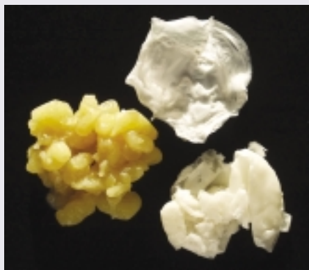
Crude extract of polyhydroxyalkanoate (PHA) before (left) and after purification (middle and right).
