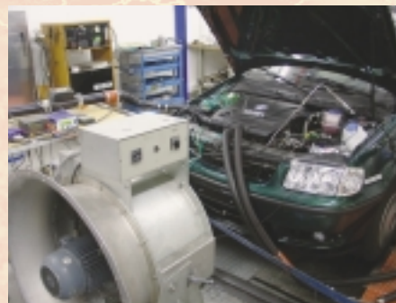
The Clean Engine Vehicle on the dynamometer
