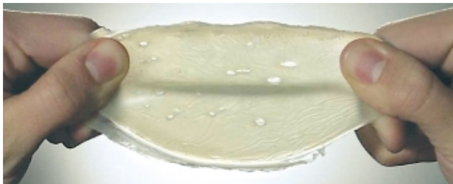
Crosslinking of unsaturated PHA allows the production of a biodegradable rubber.
