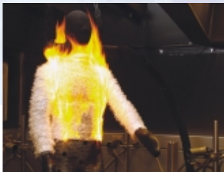
Close to real-life measurement of the effects of a clothing fire, on «Henry» the dummy. In the photograph «Henry» is being subjected to a feared «surface flash».
