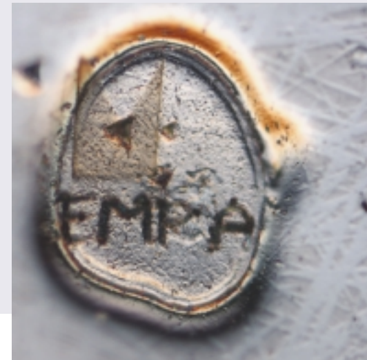
«Empa» – engraved by nanotools onto a cross-section of human hair.
