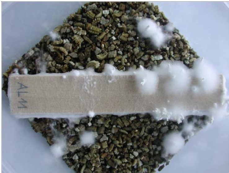
Empa test of spruce wood infected with fungi
