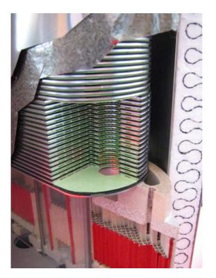
In a separate exhibition, the newest developments and prototypes from Swiss companies were on display, for example here a ceramic fuel cell stack using natural gas, with integrated gas pre-heating.
