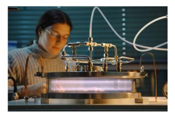
In order to combat hospital germs, medical textiles are equipped with a nanometer thick silver coating by using plasma technology. This coating considerably reduces the contamination with microorganisms. The photo shows a laboratory-experimental station at Empa.
