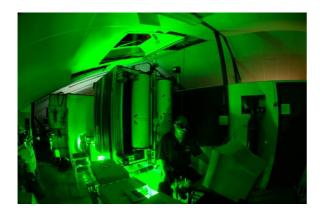
With the help of a LIDAR system, a laser radar, GEOMON researchers determine the vertical distribution of fine dust in the atmosphere.
