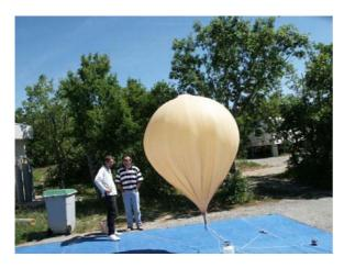
An ozone probe for atmospheric measurements is carried by a weather balloon to heights of as much as 35 kilometers; the balloon ascends from the measuring station at Haute- Provence in France. (CNRS)
