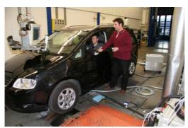
The VW Touran vehicle, retrofitted with a diesel exhaust gas filter and tested by the Empa, on the dynamometer shortly before measurements began.
