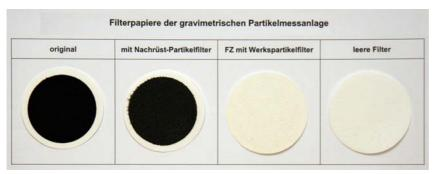
Filter papers visibly demonstrate the results of the gravimetric measurement: the exhaust gas flows through the filter paper, which holds back the soot particles. The paper is weighed before and after the test, giving a measure of the total particle mass in the diesel exhaust. With the naked eye alone one can see that the series production or OEM filter is significantly more efficient than the retrofitted device.
