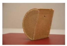
An OEM series production diesel particle filter fitted to the engine during manufacture. The filter has been cut open to demonstrate more clearly how it functions. The end of each individual channel is closed off, so the exhaust gas is forced to flow through the ceramic wall of the filter. During this process more than 95 per cent of the particulates are removed.
