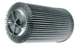
The "innards" of the tested retrofit particle filter: the exhaust gas flows through the metal filter element. In comparison to the OEM ceramic filter the metal filter is coarser, more porous and therefore much more permeable. (Image source: HJS Fahrzeugtechnik)
