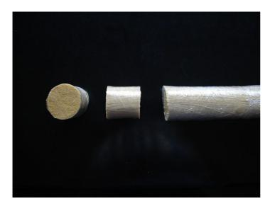
A packet that makes concrete more ductile: the newly developed fibers are supplied in a "Power Packet" that is simply added to the wet concrete. The packaging dissolves and the fibers are evenly distributed throughout the mixture.
