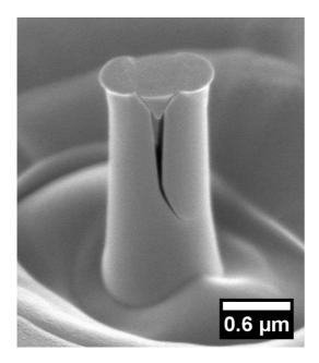
A silicon pillar with a diameter of 940 nanometers 940 after the compression test. Pillars with a diameter in excess of 400 nanometers develop cracks when loaded.
