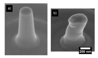
A silicon pillar with a diameter of 310 nanometers a) before loading and b) after deformation. The column has yielded to the applied force and undergone plastic deformation.
