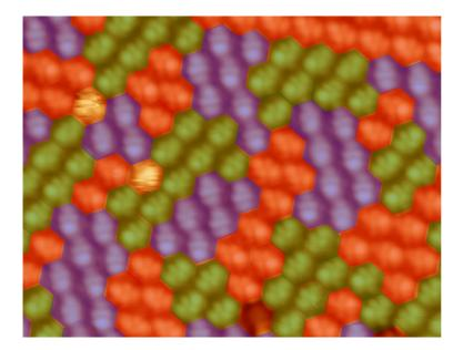
Metallofullerenes – when deposited on a surface – form ordered islands of identically orientated molecules. This scanning tunnelling microscopy image has been reproduced in colour in order to improve visual analysis – a different colour has been used for each individual orientation of the molecules.
