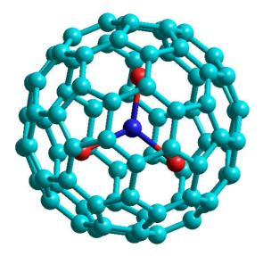
Model of the metallofullerene studied consisting of 80 carbon atoms (light blue), 3 dysprosium atoms (red) and 1 nitrogen atom (dark blue).
