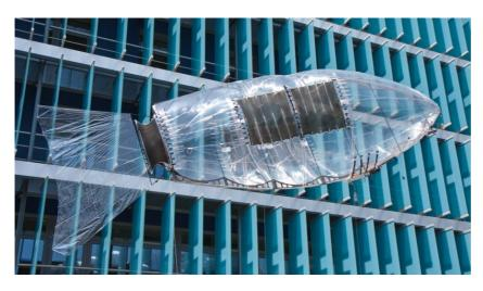
Empa's airship – the Blimp – moves like a trout through water. EAP actuators are mounted on its body and fins.
