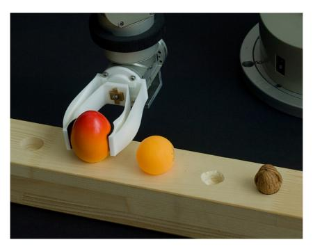
Economic tools can be made using intelligent, compliant systems. The gripping arm of this robot is made from a single molding process.
