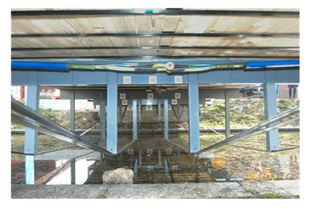
Using a video system to measure the deformation of a bowstring bridge deck made of laminated timber. The deck is tensioned by carbon fiber reinforced polymer tensioning bands spanned across the lower surface of the deck. The bands were developed at Empa.
