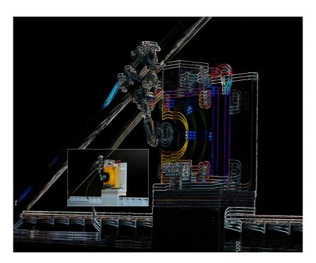
Semiactive damping system for stayed cables used in the construction of bridges. The aim is to reduce bridge oscillations to a minimum.
