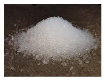
The main component of the render: aerogel, a material which consists of more than 90 per cent air.
