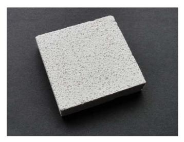
The new insulating render is simple sprayed onto walls. The photograph shows a block of the material.
