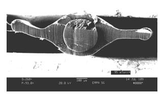
A bicomponent fiber imaged under the scanning electron microscope. The core of the fiber lends it the required stiffness whilst the sheath, of a different polymer material, gives it other desirable properties, for example optimal sliding properties.
