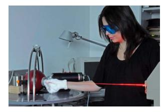
Measuring light losses in a polymer optical fiber.
