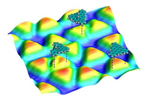
Understanding chemical reactions in detail helps to control them and enables to tailor the products. The scanning tunnelling microscope images shows nanographene molecules and the two stabilised intermediate products on a copper surface. The molecular models show a nanographene (at the bottom right) as well as the two intermediate products (above and left). In reality the diameter of the molecule is approximately one nanometre.
