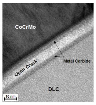
Under physiological conditions, stress corrosion cracking leads to a slow-growing crack in the metal carbide reaction layer, which is barely 5 nanometers wide. This, in turn, causes the DLC layer to detach from the implant material (cobalt-chrome-molybdenum, CoCrMo), as seen in a transmission electron microscope image.
