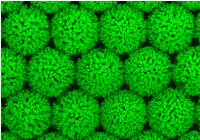
«Sea-urchins» made of tiny polystyrene balls, with zinc oxide nanowire «spines» are created using a simple electrochemical process.
