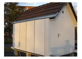
A model house on the Empa site in Duebendorf. It is fitted with façade elements treated with different plaster and paint surfaces. One surface coating contains silver nanoparticles.
