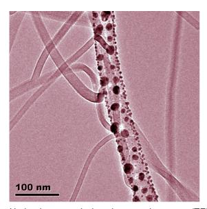
Under the transmission electron microscope (TEM): several cobalt phthalocyanine nanowires growing out of an iron phthalocyanine nanowire which is decorated with silver particles.
