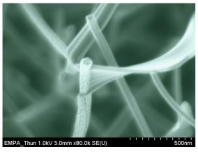
Under the scanning electron microscope (SEM): palladium octaethyl-porphyrin nano-lamellae and nanowires growing on a perylene nanowire which has been sputtered with silver particles.
