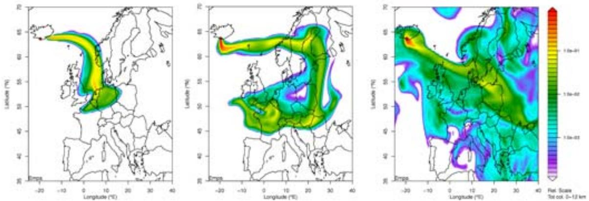
Computer simulations of ash cloud movement for 16 April (left) and 20 April (centre) and the forecast for 23 April (right)
