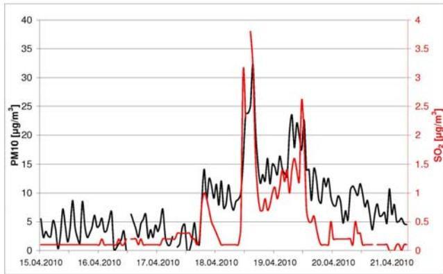
Measurements of PM10 and sulphur dioxide taken by Empa in the alpine research station on Jungfraujoch: the values increase on 18 April and fall back again on 19 April.
