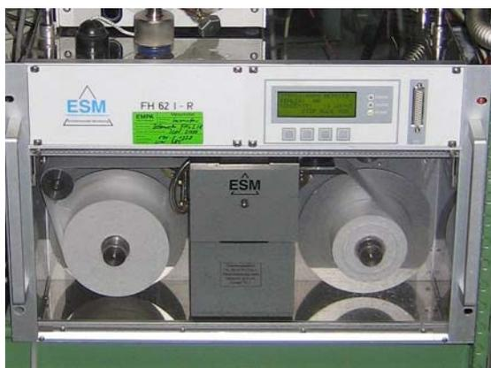
Betameter equipment used for analysing measurements of particulate matter on Jungfraujoch – a NABEL (National Air Pollution Monitoring Network) measuring station.
