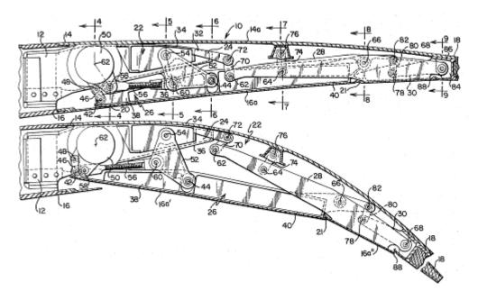
Construction drawing of a wing which adapts its shape to suit the airflow, designed using conventional mechanical engineering technologies. This kind of device was never manufactured. (US Patent, 26.01.1982, 4,312,486)
