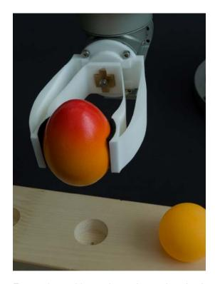
Economic machine tools can be made using intelligent, compliant material systems. The gripper arm on this robot is also manufactured from a single mold.
