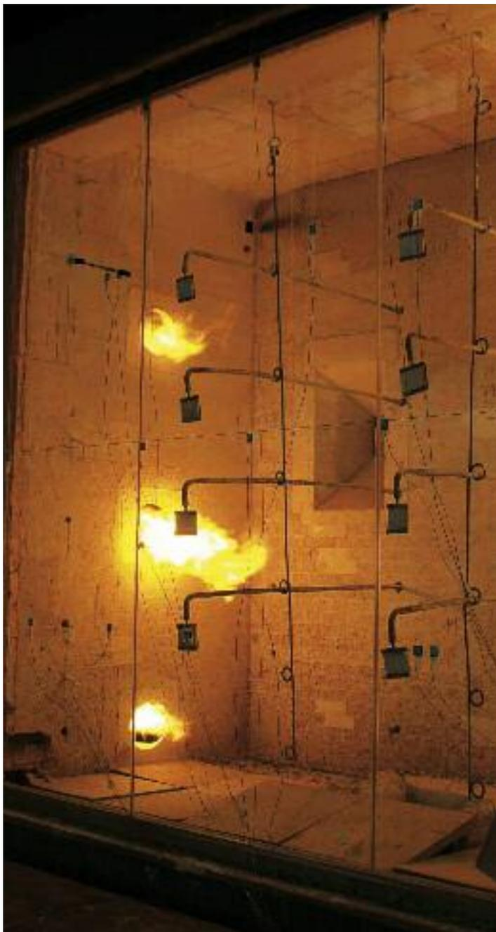
The smell of something burning tells you right away where you are. That's even before you notice the furnace in the hall, where several men are labouring to place a massive 3x3-metre pane of glass in front of it. Empa's fire specialists are placing the last deformation sensors on the glass, which is a component of a new fire-resistant glazing. Then they attach the entire testing unit – the mounting fixture including the glass – to the furnace.
