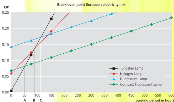
In the first 50 operating hours (European electricity mix, left) to the first 180 operating hours (Swiss mix), the tungsten lamp is, ecologically seen, still superior to its competitors. However, as the lamps burn longer, the relationship quickly changes because of the tungsten lamp's high power consumption; then the compact fluorescent lamp produces the best results. (Illustrations: André Niederer)
