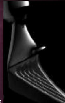
**1** The failure mechanism has been discovered – coatings made of diamond-like carbon (DLC) can detach from implants if cracks and crevices (the light area) build up in the reaction layer between the implant material and the DLC substrate.
