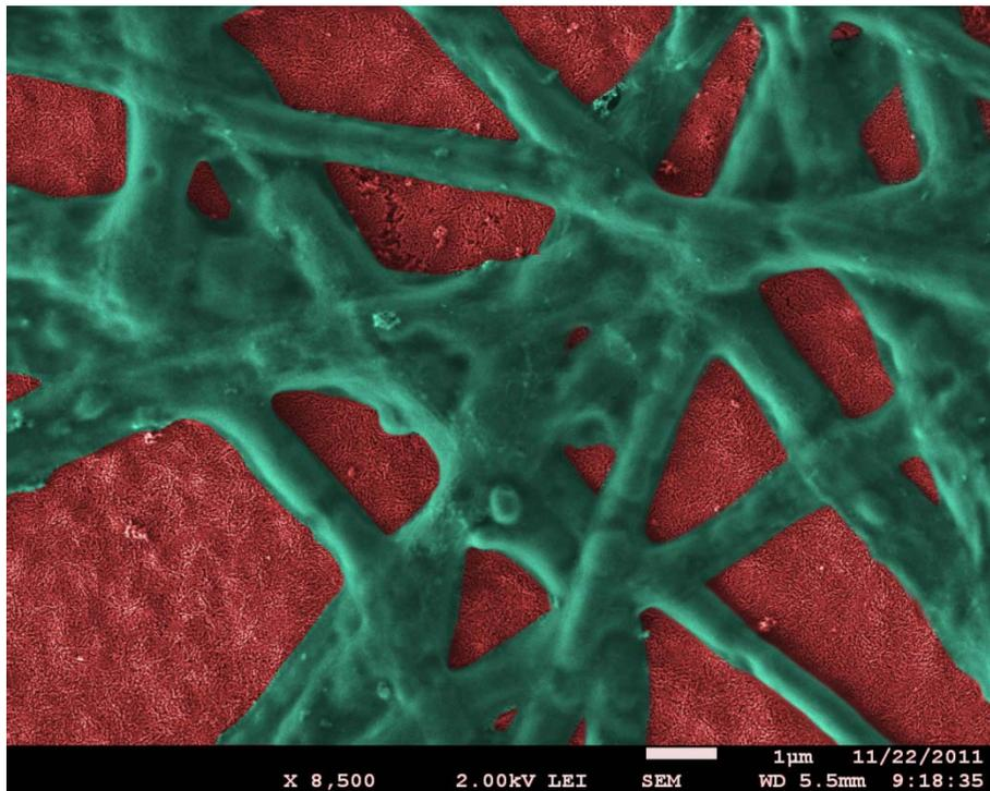
Hematite nanoparticle film (red) with functional phycocyanin network (green) attached.
