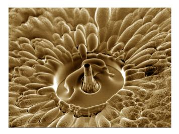
Award-winning image: Many brushes made from carbon nanotubes are formed into a tower 500 nanometres in diameter by using a focused ion beam system. The scanning electron microscope is used to investigate how they behave under the effects of pressure.
