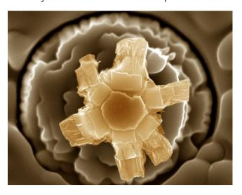
A tower made of carbon nanotubes following the stress test.
