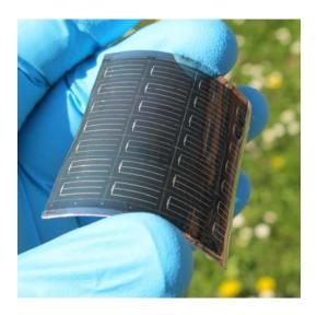
Flexible thin film CIGS solar cell on polymer substrate developed at Empa (Copyright: Empa)
