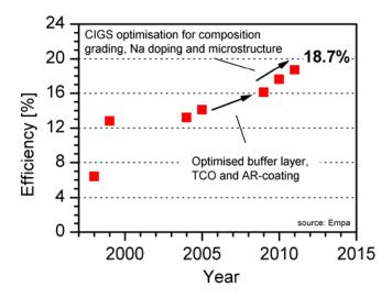
Improvement in energy conversion efficiency of flexible CIGS solar cells on polymer film
