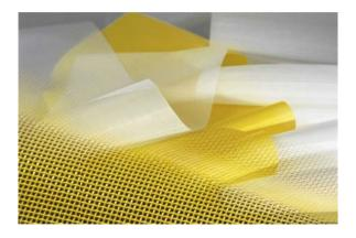
Flexible precision fabric which, in cooperation with the Swiss company Sefar AG, was developed into an electrode for thin-film solar cells.
