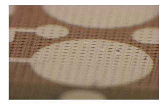
Circular organic solar cells manufactured in the laboratory. Red-brown: active organic layer; silver-grey: top electrode. Clearly visible in the photo are the woven metal wires.
