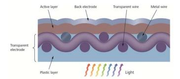
Cross-section of a thin-film solar cell with a woven electrode.
