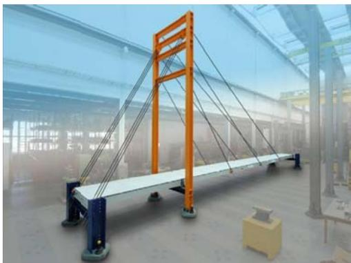
Empa will present its unique capabilities for static and dynamic surveys on large structures, e.g. a lightweight model bridge in Empa's largest laboratory. Among other uses the bridge allows scientists to compare adaptive damping elements which are used to reduce cable resonances.
