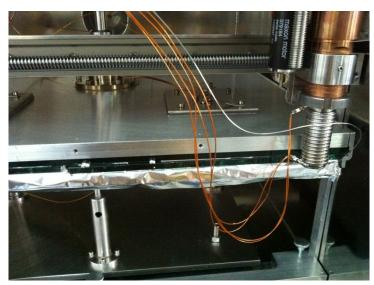
The experimental setup at Empa used to produce glazing prototypes with the new edge sealing technique. The cylindrical, copper-colored injection head is clearly visible - it injects a liquid tin alloy between the panes.
