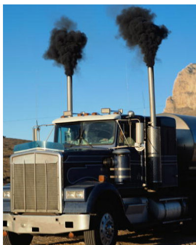
Pitch black diesel soot from the exhaust of a US truck (Image: US Environmental Protection Agency EPA)
