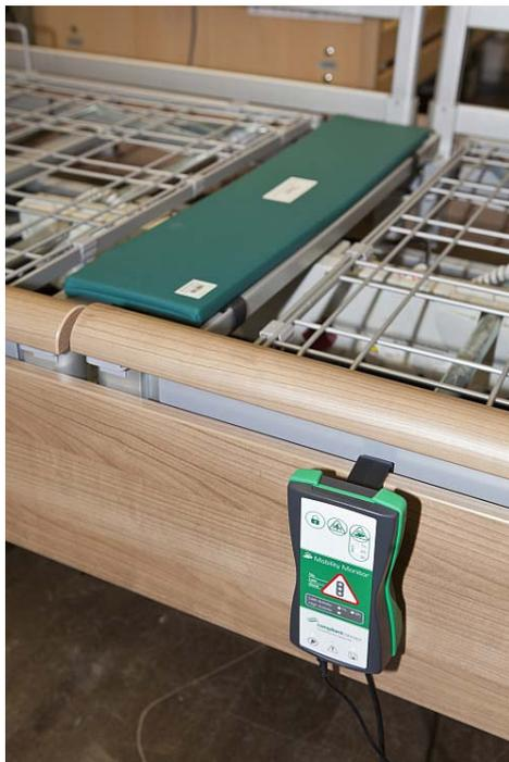
The measuring unit of the new system is installed beneath the mattress and connected to the display unit at the edge of the bed as well as to the light signaling system.
