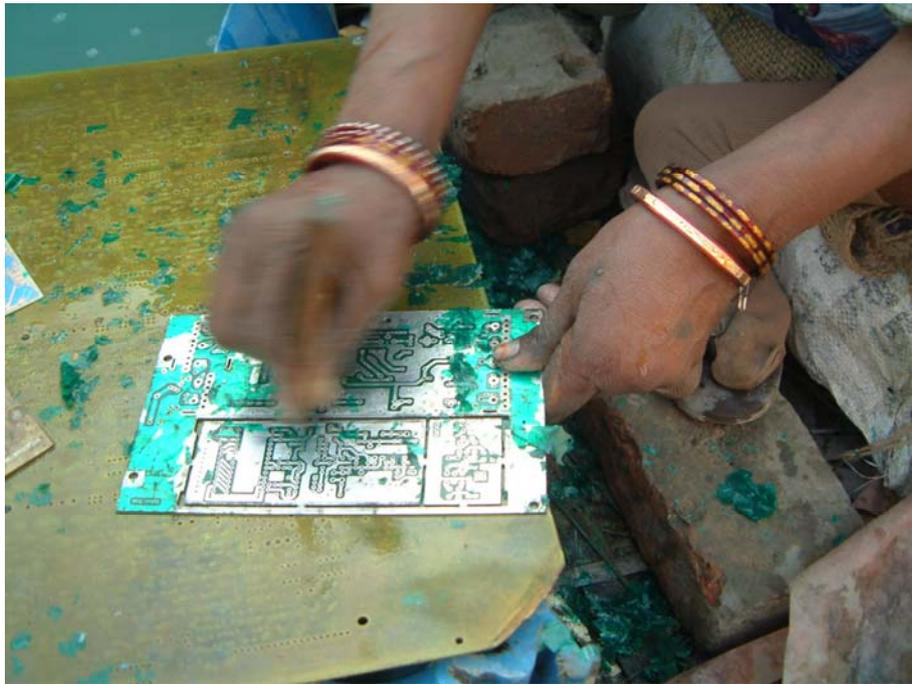
The unprofessional disassembly of electronic devices at the end of their useful life – as in this case in India, where copper is being removed from a PCB – represents a danger to human health and the environment.
