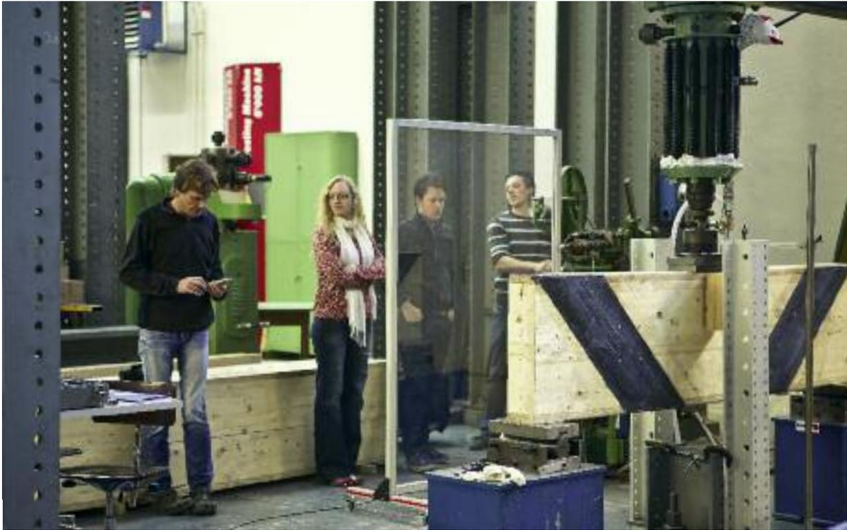
Now it gets serious: project manager Robert Widmann (left) monitors the three-point bending test on the carbon-reinforced wooden support. Engineering student Roman Frei (far right) operates the hydraulic press. At a load of 43 tonnes the laminated wood support breaks with a dull crack, and the displacement is measured. One can monitor where and when the break occurred on the computer screen.
