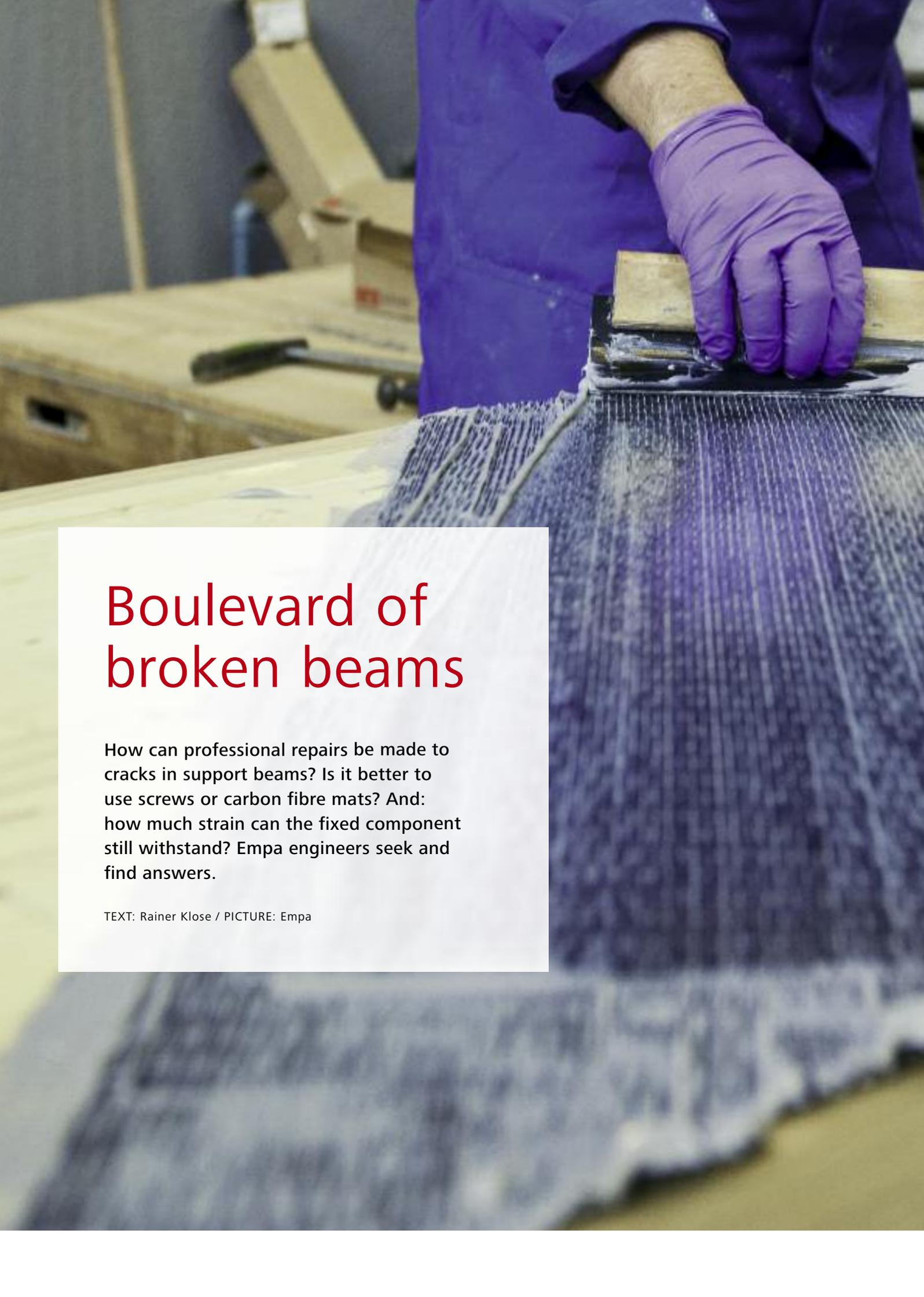
A close-up photograph of a person wearing a purple long-sleeved shirt and purple nitrile gloves. The person is using a wooden-handled tool to apply a dark, woven carbon fiber mat onto a wooden beam. The background shows a workshop environment with various wooden structures and tools.
