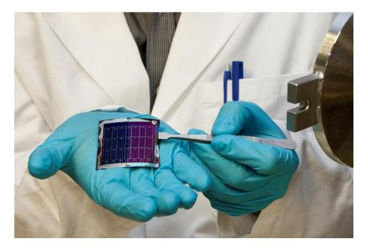
High efficiency, flexible CIGS solar cells on polyimide film developed using a new process.
