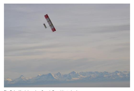
The TwingKite is based on Empa's Tensairity technology.
