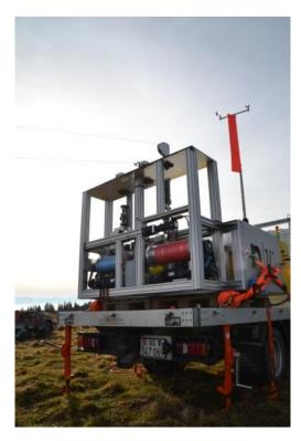
The ground station is put into position. The kite is fastened to the winders and kept in the air while the strain on them is converted into electricity.
