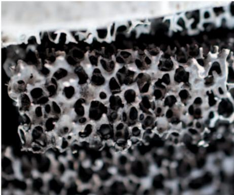
**3** The uneven structure of the ceramic foam catalytic converter creates a turbulent flow. The exhaust is evenly distributed and comes into contact with the sides much faster.
