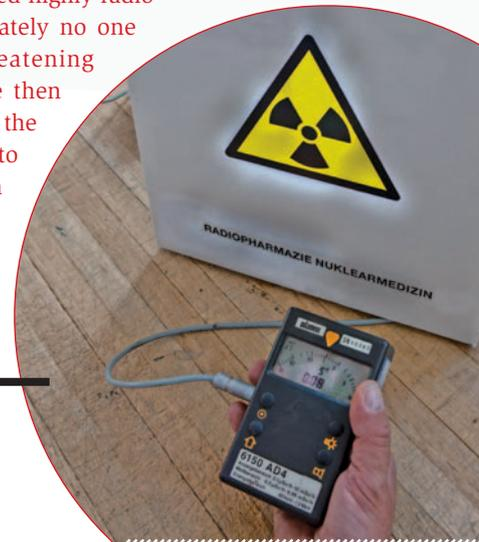
Packet checking using a Geiger counter
