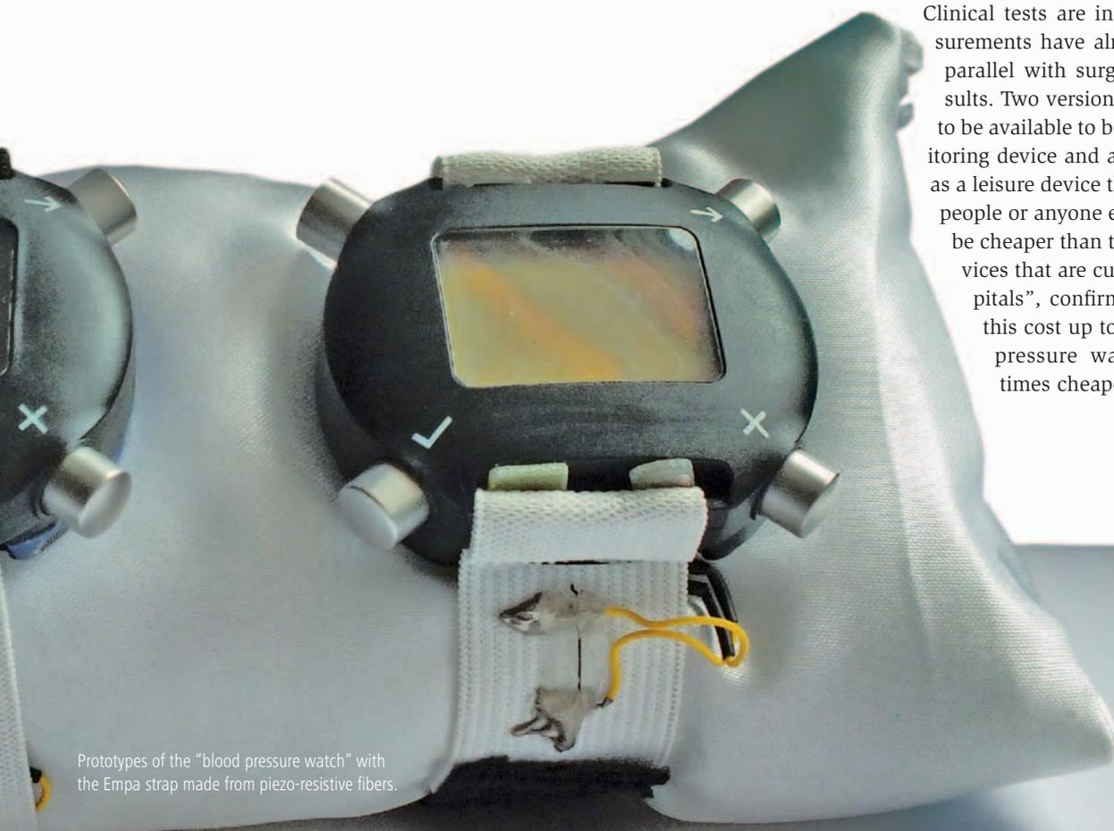
Prototypes of the “blood pressure watch” with the Empa strap made from piezo-resistive fibers.
