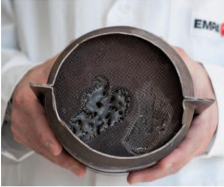
**2** This happens when hot exhaust gas flows unevenly through a conventional catalytic converter: The material melts in the hot spots. Instead of fine pores, large holes occur – the catalytic converter becomes ineffective.
