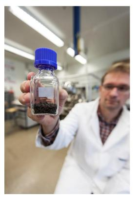
Zeolites bind the water produced during methanation of hydrogen, thereby increasing the methane yield from the new process.
