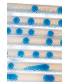
In order to make faster progress in the search for new materials, Empa has built a synthesis device in which different chemical mixtures can be produced as if on an assembly line. In the "Tubular Flow Reactor", small bubbles run through a tube in which the respective reaction always takes place under exactly the same conditions. (See p. 11.) Image: Gian Vaitl / Empa
