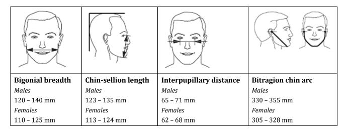
Figure 1 — Example of relevant dimensions for masks according to ISO/TS 16976-2:2015
